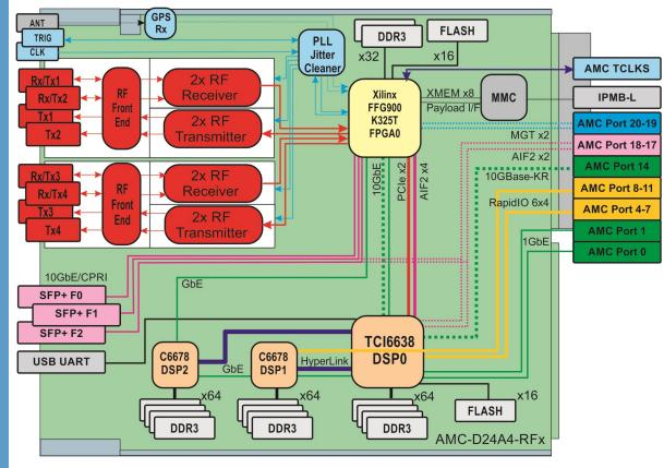
The CommAgility AMC-D24A4 is an extremely high performance ARM, DSP and FPGA based processing card which includes integrated, flexible, wideband RF transceiver channels, all in the compact double width Advanced Mezzanine Card form factor. The AMC-D24A4-RF2 has two RF channels, while the AMC-D24A4-RF4 has four.
