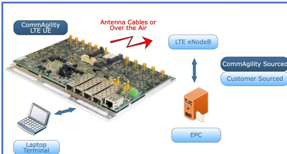
The LTE Reference UE is a pre-integrated system, including both hardware and 3GPP Rel. 10 LTE software. This flexible system is ideal for eNodeB and network testing, particularly in non-standard frequency bands.
