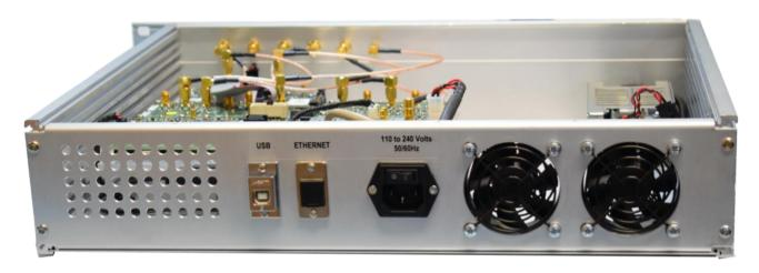
The LTE UE/eNodeB system-in-a-box is a pre-integrated solution, including both hardware and 3GPP Rel. 10 LTE software. It is available in two versions, UE and eNodeB, both based on the same hardware platform, but with different software and FPGA firmware loads.
